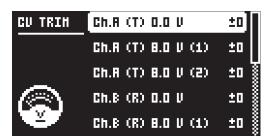
Each CV output has three trim settings. Begin by selecting 0 V, then press and hold the [YES] key. 0 V is output as long as [YES] is held down. Use [ARROW] keys [LEFT]/[RIGHT] or *DATA ENTRY KNOB A* to adjust the voltage until your voltmeter shows exactly 0 V. Repeat the process for both 8 V settings (the first one is for continuous voltage, the second is for pulse).
