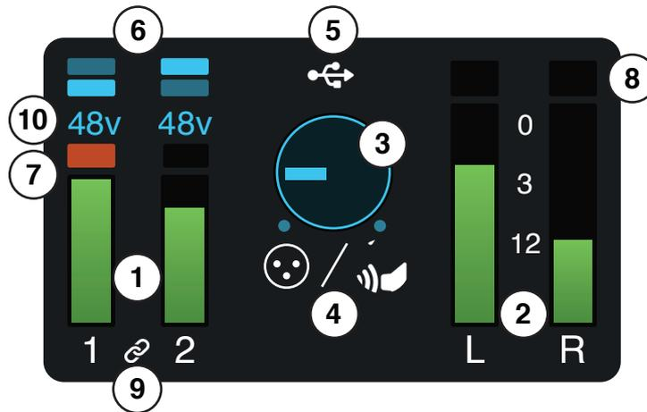
1. **Input Meters.** These meters indicate the input level of the analog inputs on your Revelator io24. The red Clip indicator will light when your input signal reaches -0.5 dBFS. At this level, the signal will begin to overload the analog-to-digital converters and exhibit signs of clipping. Use the gain controls to keep the signal below this level.
