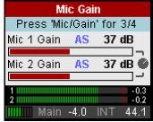
As soon as AutoSet reduces the gain the label AS, shown in the front display, changes its colour from black to blue.
