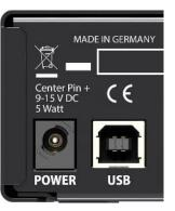
**Power**. Serves to unload the computer's power supply or to ensure power delivery in case it is not sufficient or fails on the computer side. In principle, the device also works without a power supply (USB buspowered).
