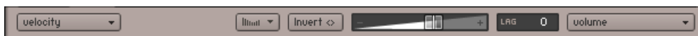
An external modulation assignment which maps MIDI Velocity to the volume parameter of an Amplifier Module.
