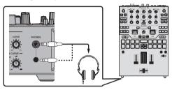
2 Connect devices such as powered speakers, a power amplifier, and components to the [MASTER 1] or [MASTER 2] terminal.
