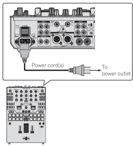
6 Press the [POWER] switch on this unit's rear panel to turn this unit's power on.
