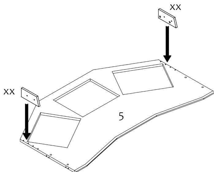
STEP 2 Put the desktop n° 5 face down, flat on the ground. Using assembly kits add the two parts XX on either side.
