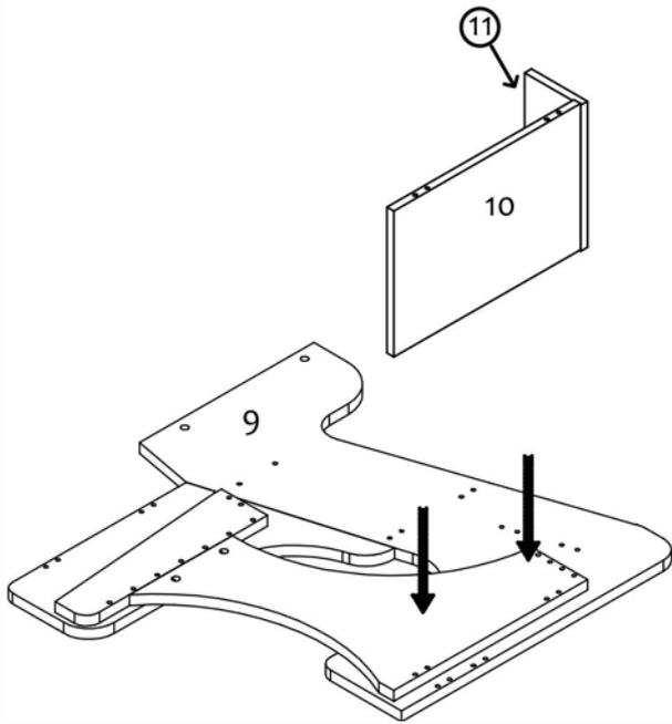
STEP 5 Lay side part n° 9 face down on the ground (we recommend using carpet or soft surface to avoid scratches) and lower down the parts n° 10 and 11 and fixate using wooden pegs.
