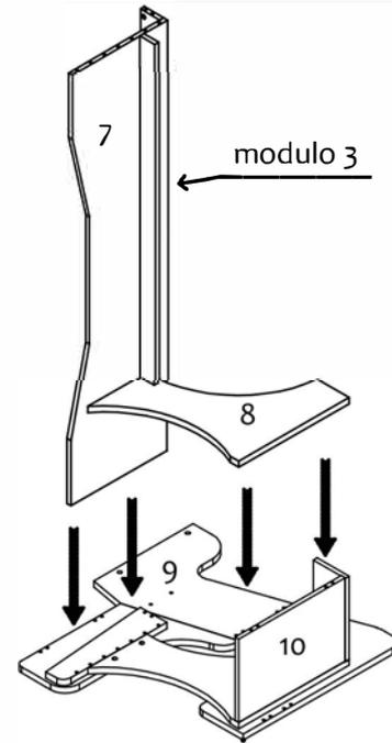
STEP 6 Add more bolts. Lower down module 3 onto parts n° 9 - 10 - 11 previously assembled. Be careful to align all the bolts and holes and fix using excenters.
