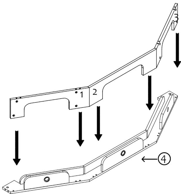
STEP 1 (module 1) Put part n° 4 down flat and add system bolts (page 2), lower down parts n°1 ,2+ 3. Fixate using the excenters as shown in page 2.
