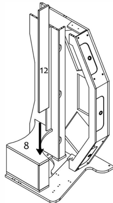
STEP 8 Fixate part n° 12 to part n° 8 aligning bolts and holes and tighten with excenters.
