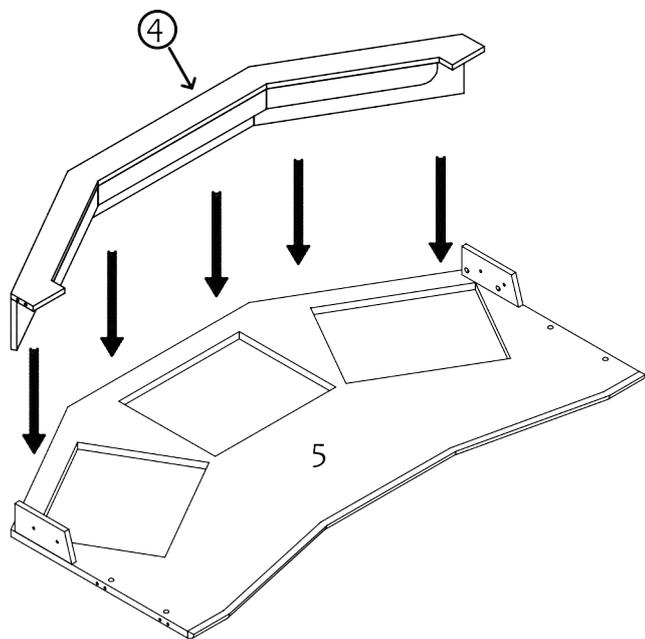
STEP 3 (module 2) with desk top n° 5 still lying flat, add the cable tray (module 1) previously assembled using the assembly kits as shown in page 2.
